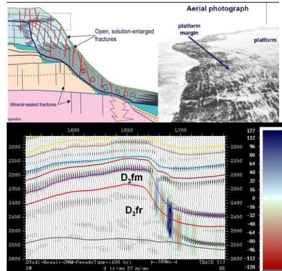
Figure 6: Top left – the principal model of the carbonate platform edge with network of syndepositional fractures (Narr W. et al., 2008). Top right – photo of an outcropping (Playford P.E et al., 1984), below – the color-coded section of the duplex wave amplitudes' field with conventional seismic in wiggle.
