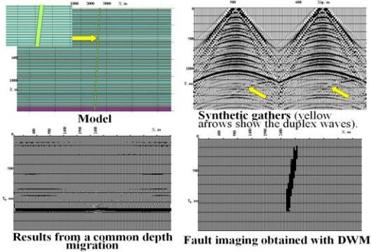
Figure 2: Seismic imaging of low throw faults in a horizontally layered medium.
