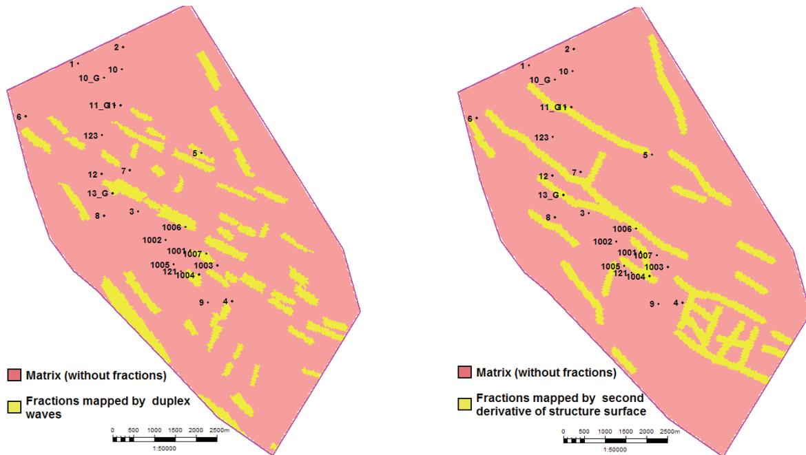
**Figure 1.** Maps of the fractured zones in the static model. Left) Using DWM method. Right) Using method of the second derivative.
