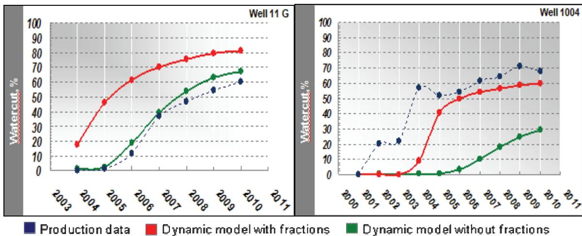
**Figure 2.** Observed (blue) water cut in selected wells vs. water cut in the same wells on model without fractures (green) and with fractures predicted with DWM method (red)
