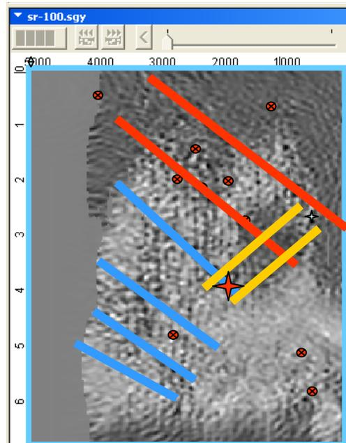
Figure 3: a) Depth slice of coherency cube computed from conventional PSDM. b) Aeromag survey with DWM interpreted faulting. c) Depth slice of 1 of 4 DWM cube views. d) Interpreted DWM depth slice – red indicates faults intruded with igneous rocks, blue and yellow indicate parallel and orthogonal faulting common in area.
