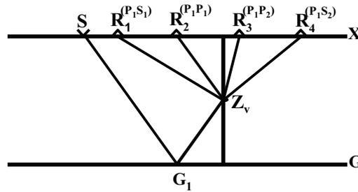
Figure.1 Scheme of the formation of four types of duplex waves at a vertical boundary.
