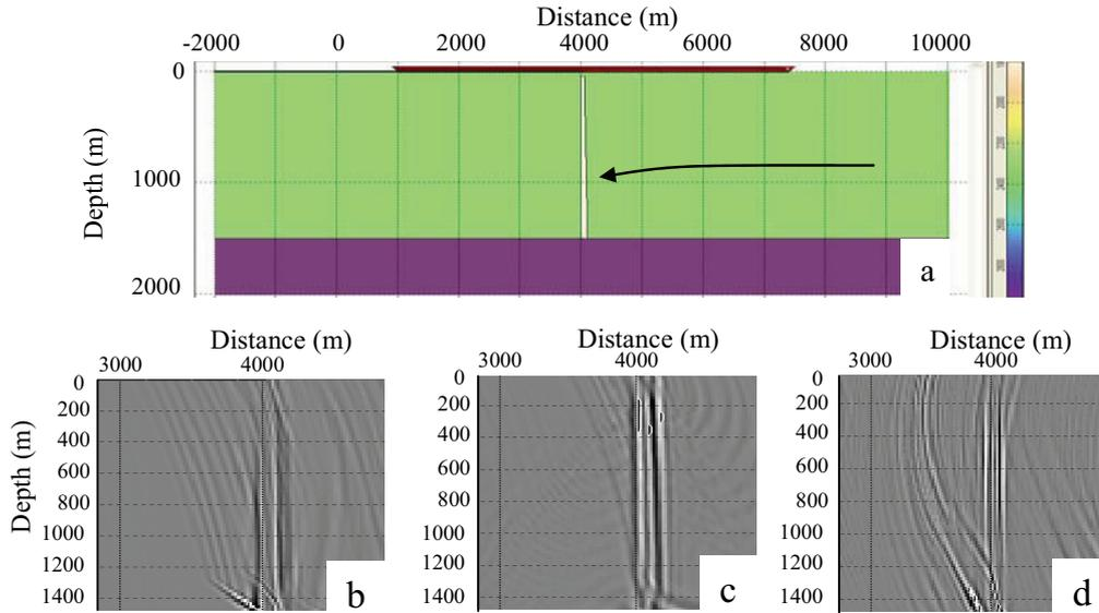
Figure 2. Image of a thin vertical dike obtained with different types of duplex waves. Model (a); images obtained with: compressional reflected wave (b), transmitted converted wave (c); reflected converted wave (d). The dike of a 80 m thickness is marked with the arrow.
