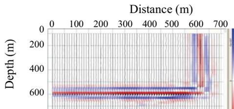
Figure 4. Image obtained with TWFM. Primary reflections as well as duplex compressional and converted waves were used.
