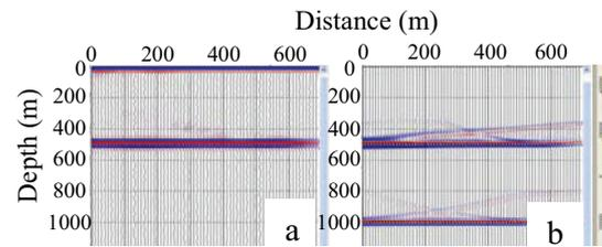
Figure 5. Images obtained with primary and multiple reflections: TWFM (a) and Kirchhoff migration (b).
