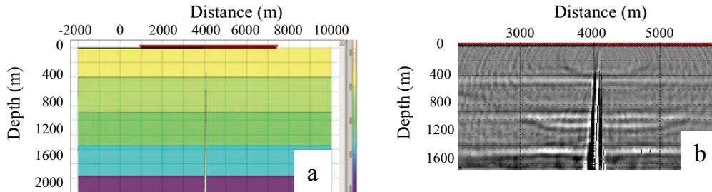
Figure 3. Model of a dike thinning to the top in a horizontally layered medium (a) and image obtained with transmitted converted duplex waves (b). The image contains both horizontal and vertical boundaries.
