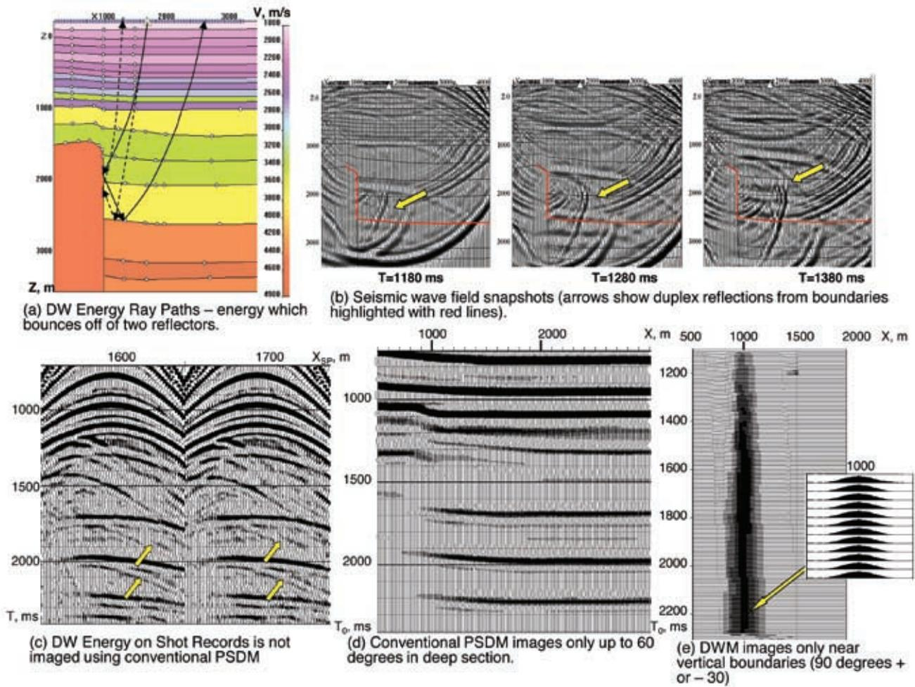
**Figure 2** Comparison of imaging capabilities of conventional PSDM versus DWM. (a) Duplex wave energy raypaths for energy which bounces off two reflectors. (b) Seismic wavefield snapshots (arrows show duplex reflections from boundaries highlighted with red lines). (c) Duplex wave energy on shot records is not imaged using conventional PSDM. (d) Conventional PSDM images only up to 60° in the deep section. (e) DWM images only near vertical boundaries (90° ± 30°).
